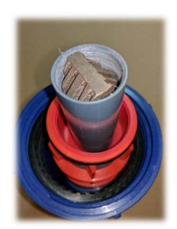
2. Using a funnel if necessary, pour 10.5 oz of poly-phosphate crystals into the filter. Do not overfill which will keep the red top cap from fitting all the way
