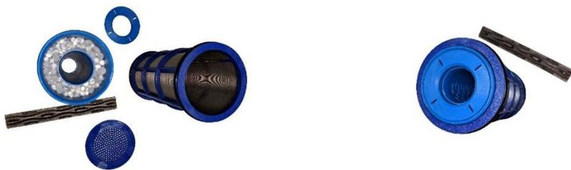
Approximately every 8-10 months, check the level of poly-phosphate and you can remove and clean the Hard Water Bullet catalytic core and clean the 50-mic filter at this time if needed using a tooth brush **from the inside out.**
